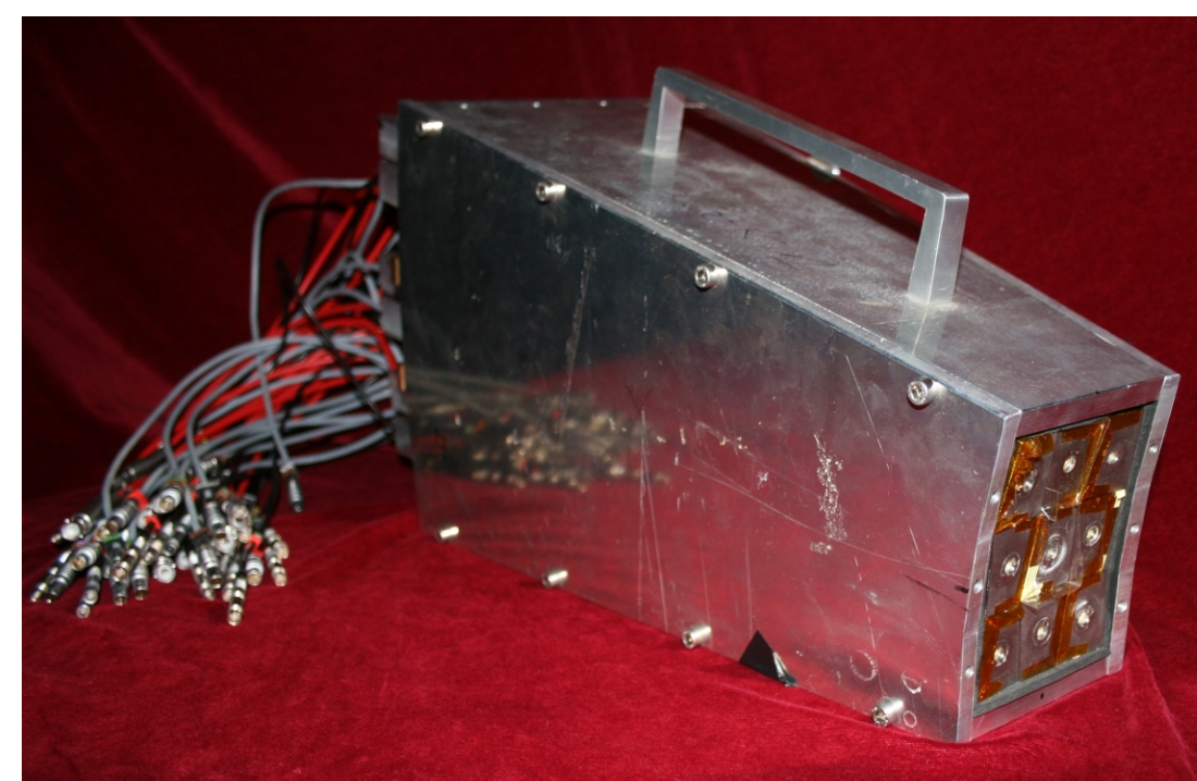
3x3 matrix of CsI(Tl) crystals
