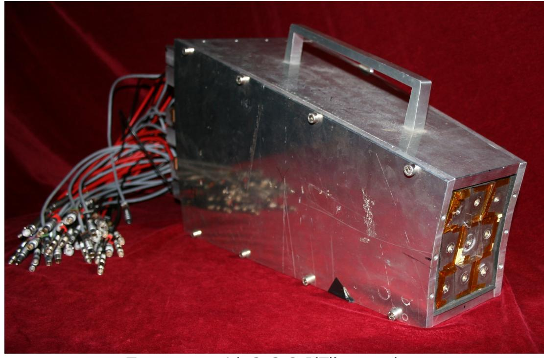
Test setup with 3x3 CsI(Tl) crystal array.
