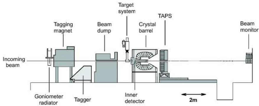
**FIGURE 1.** Experimental setup of CBELSA/TAPS in Bonn. The electron beam delivered by the accelerator ELSA enters from the left side and hits the diamond crystal of the goniometer.
