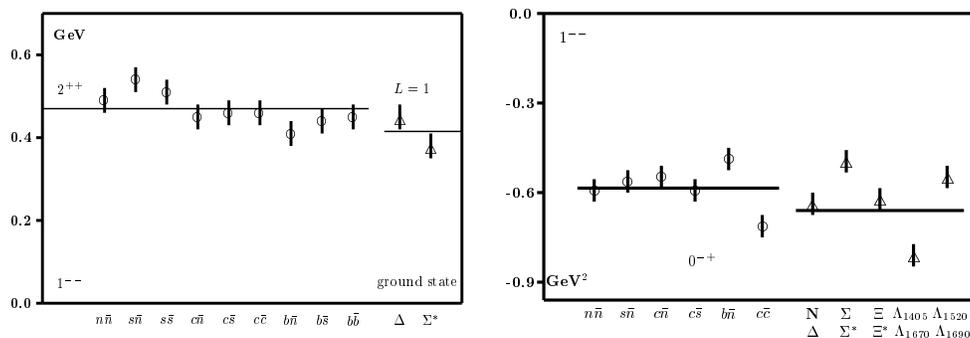
**FIGURE 1.** Flavor independence of the strong forces: Left panel: Mass differences for  $L = 1$  excitations of mesons and baryons (for systems with aligned spin). Right panel: Mass square differences between PS and V mesons for  $L = 0$  octet-decuplet and  $L = 1$  singlet-octet baryons.
