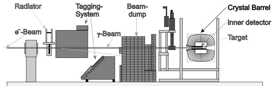
Figure 1. Experimental setup at ELSA in Bonn
