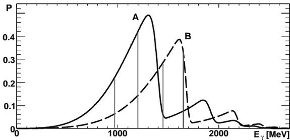
**Fig. 1.** Degree of linear polarization for the two different settings. Maximum degrees of polarization were 49.2% at  $E_\gamma = 1300$  MeV (A) and 38.7% at 1600 MeV (B) respectively (see [5] for details). Vertical lines indicate the energy ranges under consideration.
